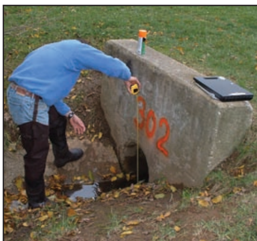
Figure 27: Measuring Outfall Diameter
