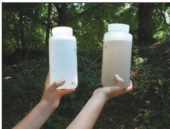
Figure 33: Using a sample bottle to estimate color and turbidity
