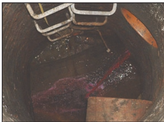
Figure 64: Dye in a mesh bag is placed into an upstream manhole (left); Dye observed at a downstream manhole traces the path of the storm drain (right)
