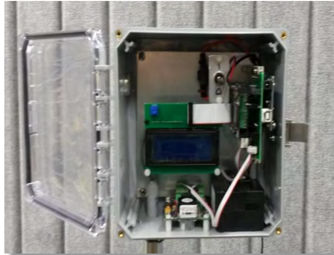
CSAM with sensors and built-in micro-computer
