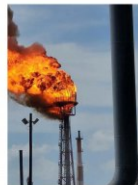
Air pollution from an improperly operated flare
